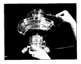
Take the weight of the fan and offer the canopy up to the mounting plate. Two keyed slots in the canopy will align with the two screws that have been left in the mounting plate.
