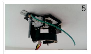
The final position of the nuts is shown on the left. The bracket is now firmly secured to the Big Strip Fastener
