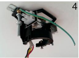
Note that the big strip fastener is supplied with 2 sets of nuts. They are identical but the second goes in behind the first as a locking nut.
