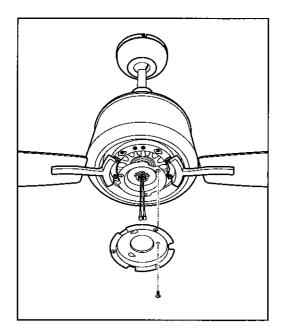
Remove one of the three light plate screws from the mounting ring and loosen the other two screws. (Do not remove.)
