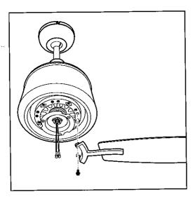
Align the holes from the blade holder to the holes from the motor, and secure the blade holder in place with screws and washers provided. Repeat this process to attach the other blades assemblies.
