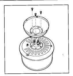
Release 3 screws from upper housing, put the canopy onto the drop rod boss of the fan. Using the 3 upper housing screws to screw the canopy tight. Please refer to the pictures .
