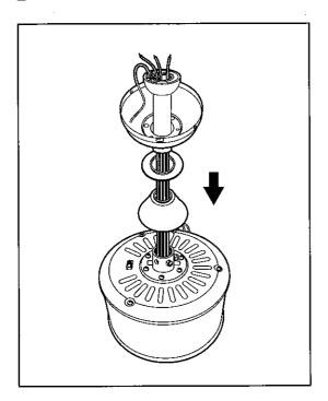
Remove the cotter pin and cross pin from the drop rod boss of the fan. If a longer drop rod (12" to 72" rod) is going to be used transfer the ball joint and the earth wire to the longer rod.
