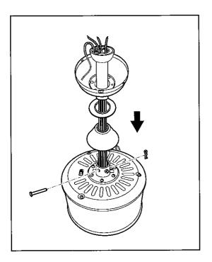
Loosen the drop rod set screws on the boss, which is on top of the motor and insert the drop rod into the drop rod boss on top of the motor casing. Turn gently to align the holes in the boss with those in the rod. Ease the split pin through the boss and the rod taking care not to pinch or damage any cables. Fix in place by replacing the cotter pin.
