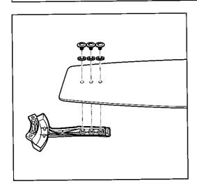
Attach the blade to the blade holder using the three blade set screws and fiber washers. Start a screw with fiber washer into the blade holder, but do not tighten. Repeat for the two remaining blade set screws and fiber washers.
