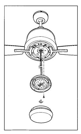
Remove one of the three light fitter screws from the light plate and loosen the other two screws. (Do not remove.)
