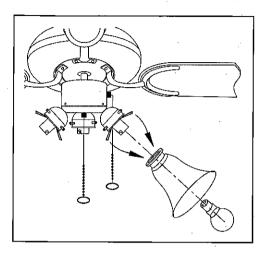
Your unit has been supplied pre-fitted with a light kit, mount the glass shades onto the light fitting using the spring clips and secure in place with the thumb screws provided.
