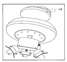
Take the weight of the fan and offer the canopy up to the mounting plate. Two keyed slots in the canopy will align with the two screws that have been left in the mounting plate.
