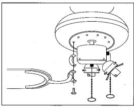
Using the motor screw and the spring washers provided, bolt the carrier bracket on to the motor. Ensure the bolts are tightened firmly.
