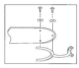
The blades now need to be assembled on to the carrier brackets.
