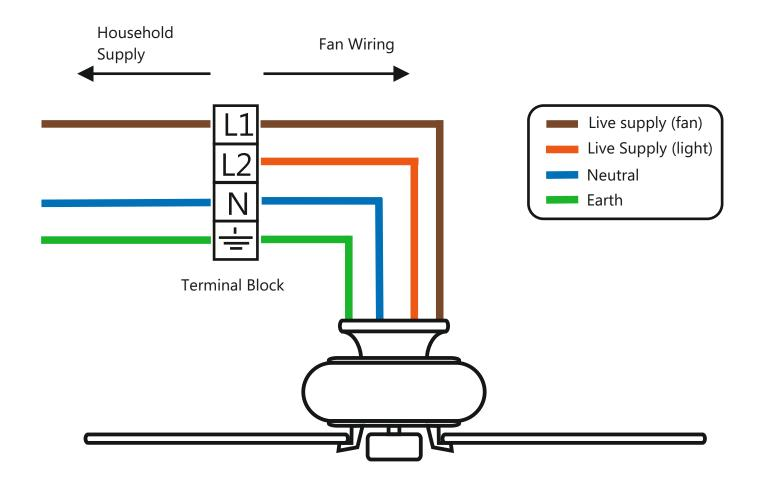
Note: If a light is planned at a later date then connect Brown and Orange wires to L1
