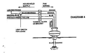
5. Wall switch operating the fan, pull switch operating the light.
