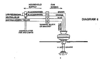
Do not connect the motor supply cable to a dimmer switch. If a wall mounted control for the fan is required then we recommend you contact our help-line.
