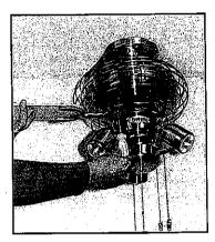
Using the coarse threaded short bolts and the spring washers provided, bolt the carrier bracket on to the motor. Ensure the bolts are tightened firmly.
