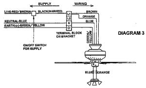
Wall switch operating the light, pull switch operating the fan.
